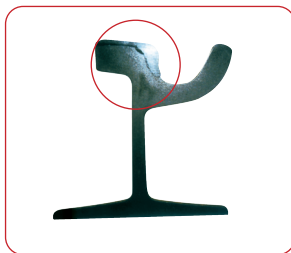
Macrostructure of top and side rail weld
